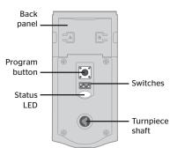
Note: When the cover is removed, the turnpiece shaft can be used to manually lock and unlock the door.
